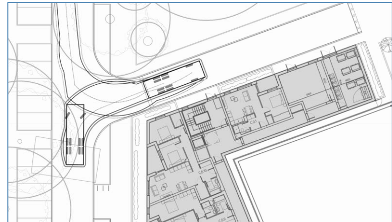
Figure 7: Extract of GF displaying Refuse 3 Axle Turning Radius | NTS
